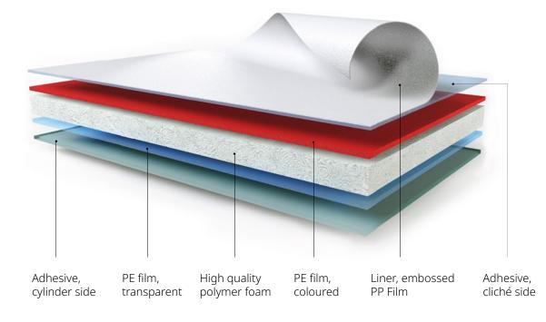
The **ORAFLEX**<sup>®</sup> Cushion Tapes' compressible foam and film reinforcement construction technology guarantees an optimized thickness accuracy, with minimal thickness tolerances (+/- 0.02 mm).
