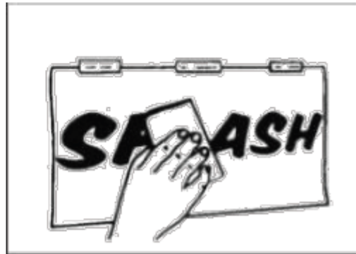
6) After two minutes either saturate transfer tape with SPLASH or proceed with dry removal of transfer tape.
