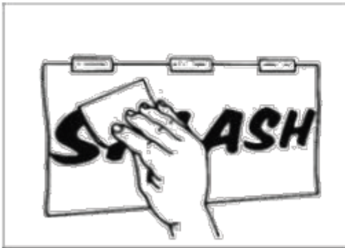
5) Lay copy on wet surface, position squeegee down.
